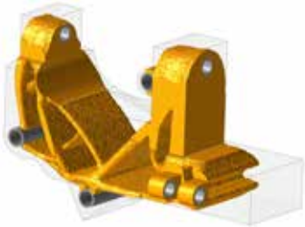
Trunnion bracket concept generation: Multiple parts can be defined as design space
