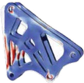
Bell Crank final design von Mises stress analysis
